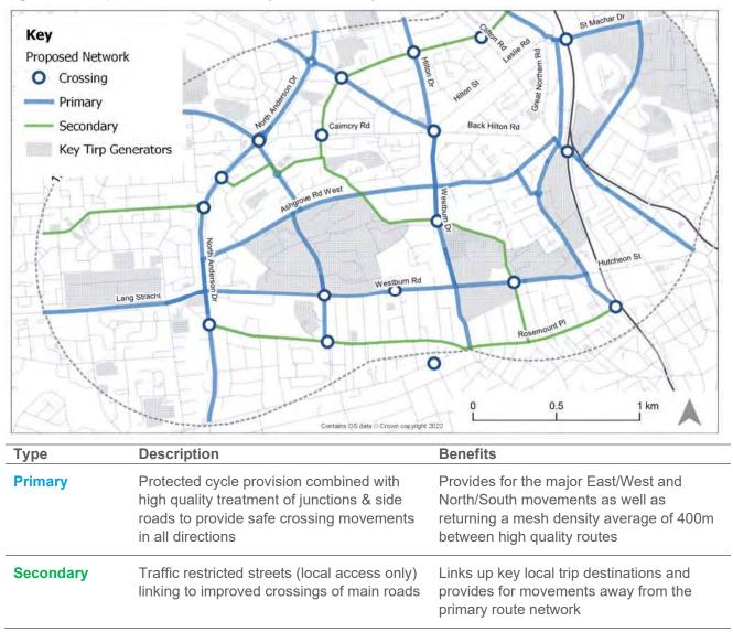
Figure 6.3: Proposed Network of Primary and Secondary Routes
